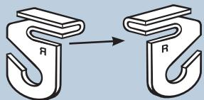
Create an open hook using a Left Hook and Right Hook (L+R)
